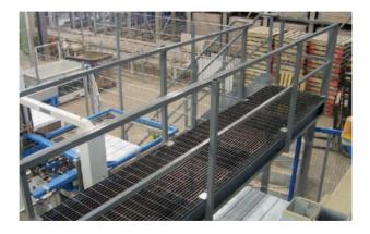
It is a types of platform grating ensuring worker's safety against any items that makes surfaces slippery in the working environment.
